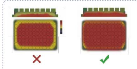
Using the latest generation of imported semiconductor technology, excellent amplification performance, effectively eliminating the edge effect of heat conduction of the block, and excellent temperature uniformity of the block.
